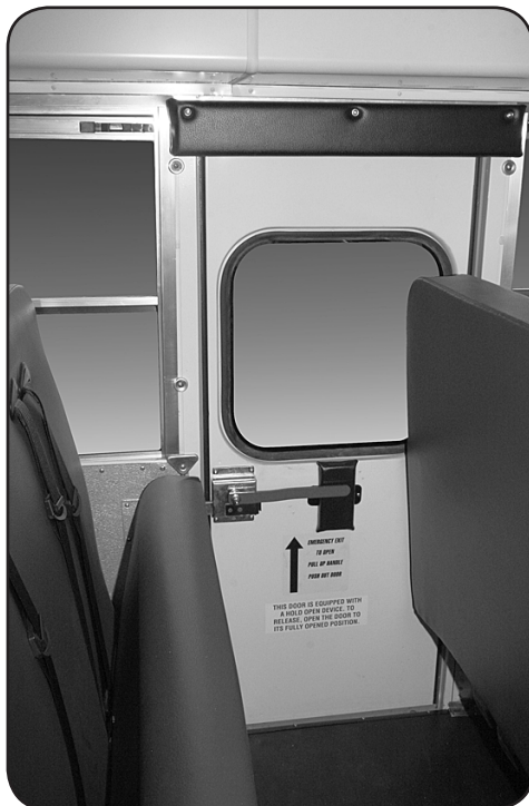
Side Emergency Door
