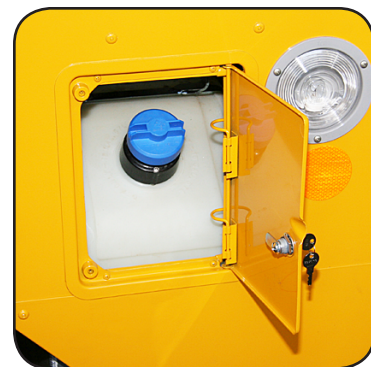
DEF Fill located to the left of the entrance door.
