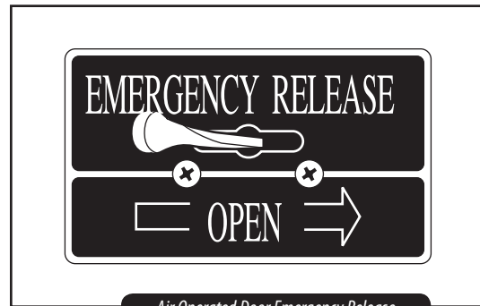
Air Operated Door Emergency Release
