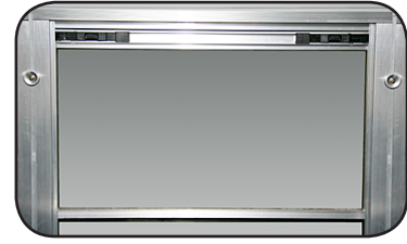
Push inward on both slide latches to lower window.
