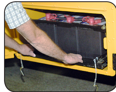
... and slide the battery tray outward.
