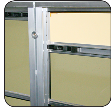
Each window has five open positions. When in any of the top four positions, the window sash can be closed (raised) without retracting the latches.
