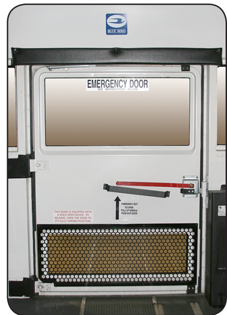
Rear Emergency Door
