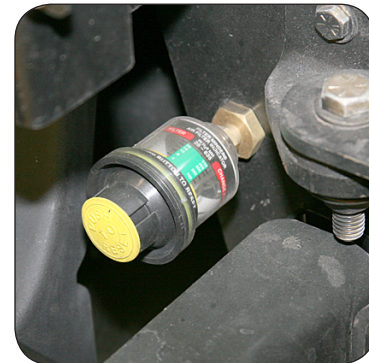
Air Restriction Indicator behind Front Left Access Panel
