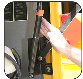
Engine Access Door Prop Release Push in to close engine access door
