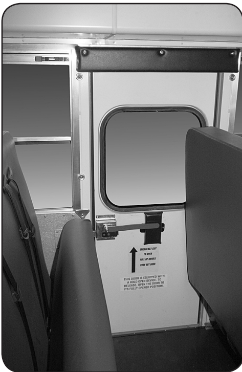
Side Emergency Door
