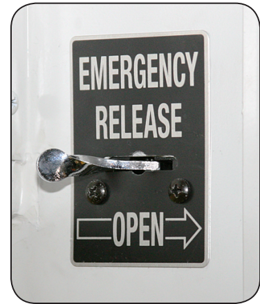
Air Door Emergency Release
