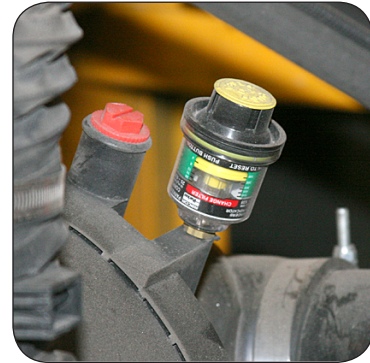
Air Restriction Indicator at Air Intake Filter Element
