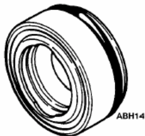
Inspect Shaft Seal
