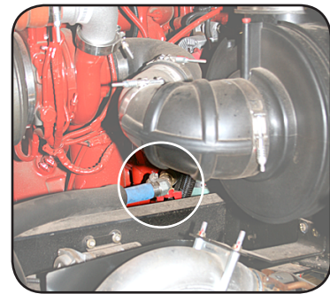
Rear Engine heater return cutoff valve. Accessible from under the bus, forward of the radiator.
