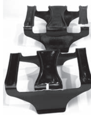
FIGURE 7-16 Axle Wrap Liners Unacceptable Cracks
