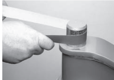
FIGURE 9-53 KINGPIN AFTER CLEANING
