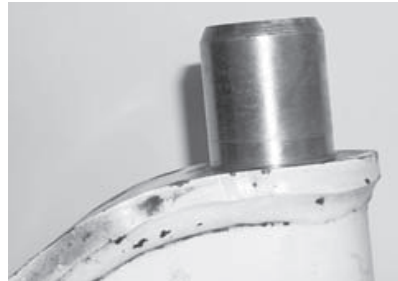
FIGURE 9-53 KINGPIN AFTER CLEANING
