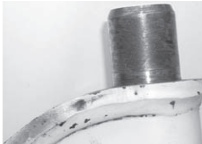
FIGURE 9-52 KINGPIN BEFORE CLEANING
