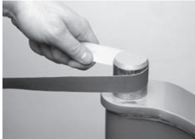
FIGURE 9-52 KINGPIN BEFORE CLEANING
