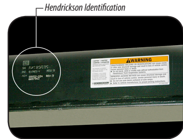
The specific Hendrickson axle model installed may be identified by referring to the axle numbers etched near the center front of the axle's main beam.
