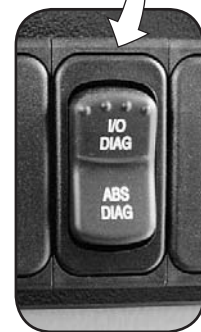
Diagnostic Mode Switch Cycles the MBC's display through Ports, Inputs, Outputs, and Feedbacks. (3-position momentary)
