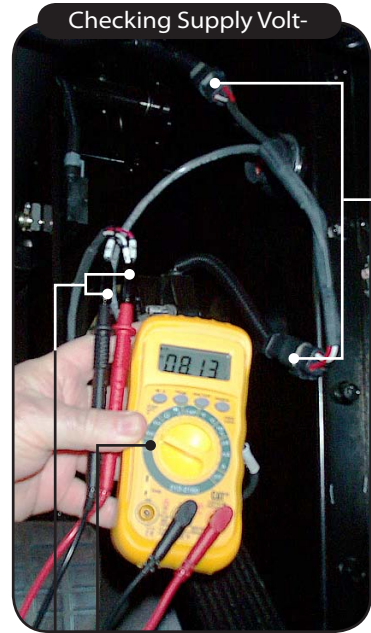
Meter set to read Volts DC.
