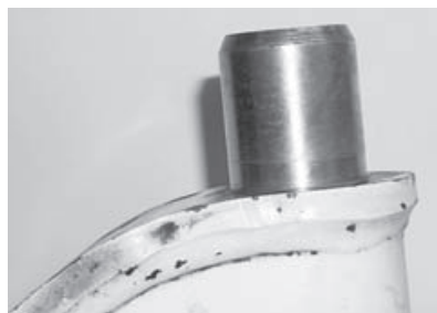
FIGURE 9-55 KINGPIN AFTER CLEANING
