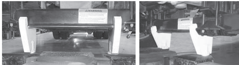
FIGURES 6-2 AND 6-3 PROPER TOW FORK LOCATION ON INSIDE CLAMP GROUP ON THE STEERTEK AXLE
