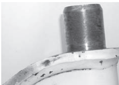
FIGURE 9-54 KINGPIN BEFORE CLEANING
