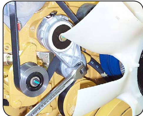
Turning the tensioner to allow belt removal.
